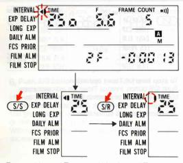
To cancel Interval Timer set during Interval Timer operation, push S/S button, then push S/R button.
